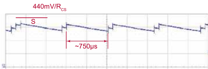
Fig.2. Short-circuit inductor current.
